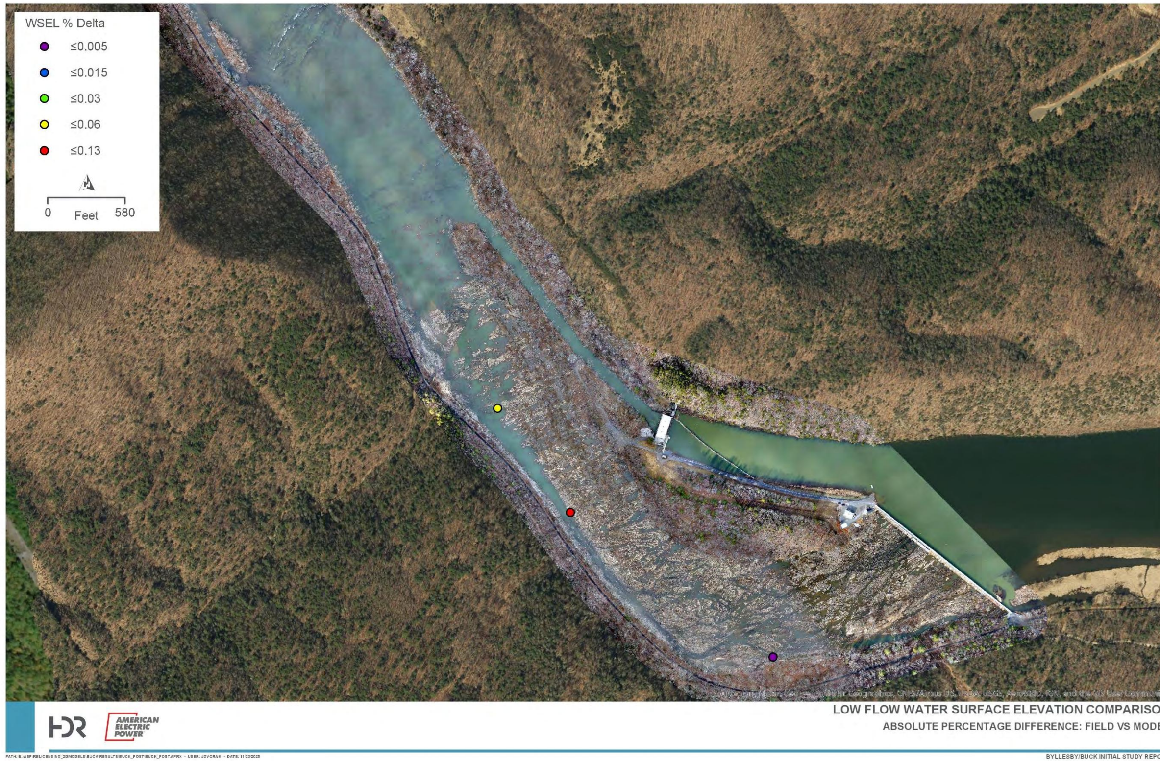
Figure 4-2. Field vs Modeled Water Surface Elevations – Day 2 (Low) Target Flow
