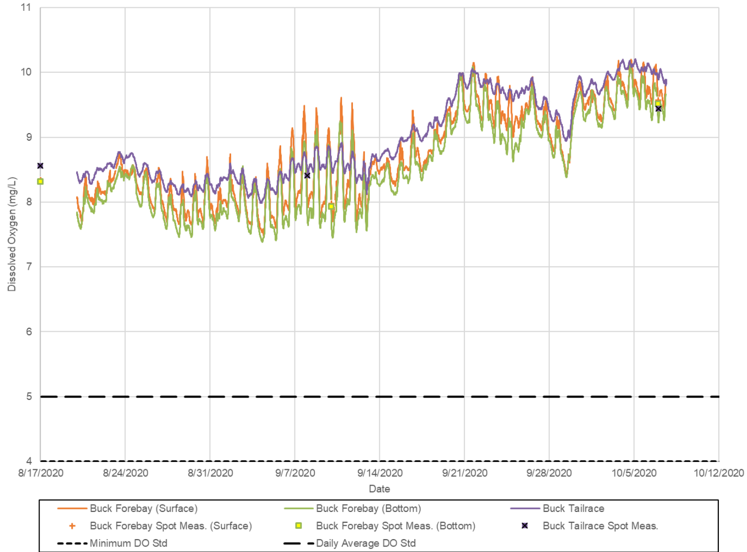
Figure 1-5. Continuous and Discrete Dissolved Oxygen Concentrations at Buck Forebay and Tailrace Water Quality Monitoring Locations
