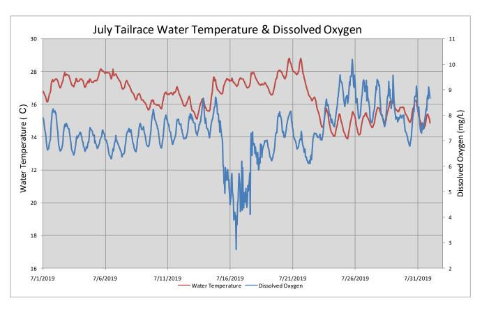
\*Tailrace logger data had two instances where the DO readings were suspect. These instances were from June 12-21, 2019 and from July 14-19, 2019. These were possibly due to turbulence or shock from upwelling at this location. No secondary logger data was available for comparison due to a malfunction with the secondary logger.
