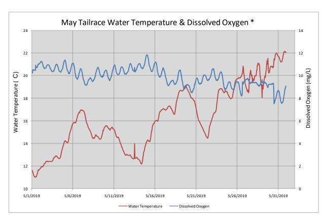
\*On or around May 21, 2019, it is suspected that both loggers in the tailrace were pushed up onto the concrete ledge due to upwelling. The primary logger was damaged during this action and quit recording on May 21 while the secondary logger continued to record data from what could have been a position above the water. Because of the damage to the primary logger, data from the secondary logger was used for the month of May. The primary logger was replaced on May 30, 2019.
