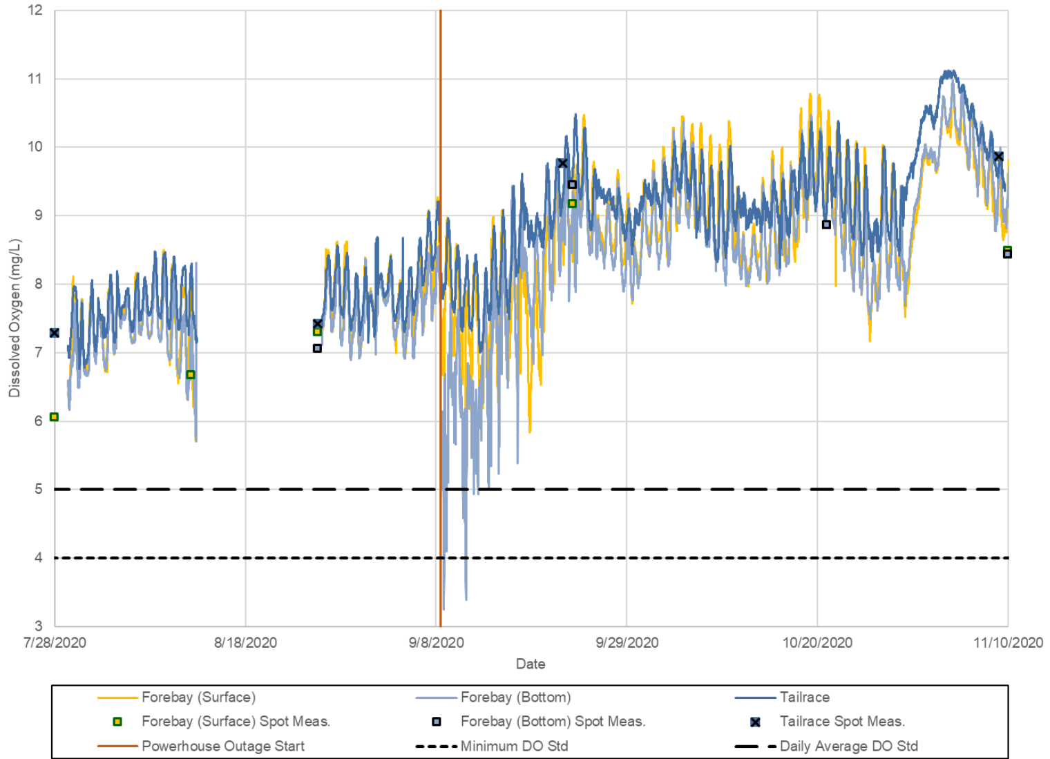
Figure 1-3. Continuous and Discrete Dissolved Oxygen Concentrations at the Forebay and Tailrace Water Quality Monitoring Locations
