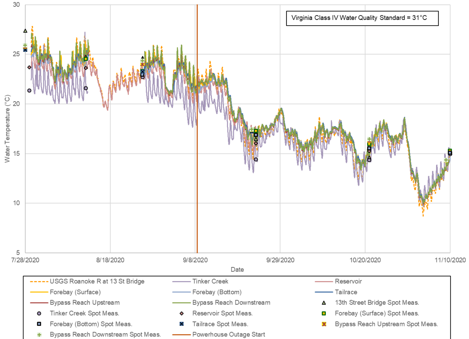
Figure 1-1. Continuous and Discrete Temperature Measurements at All Water Quality Monitoring Locations
