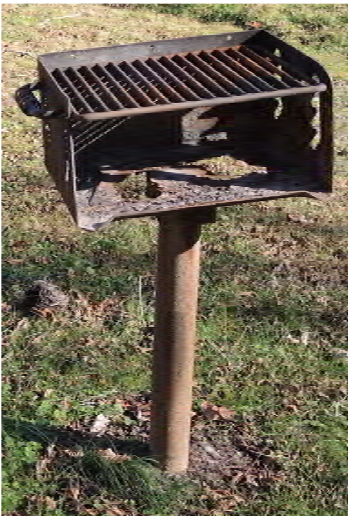
Photo 5-6: BBQ grill with rusted out bottom
