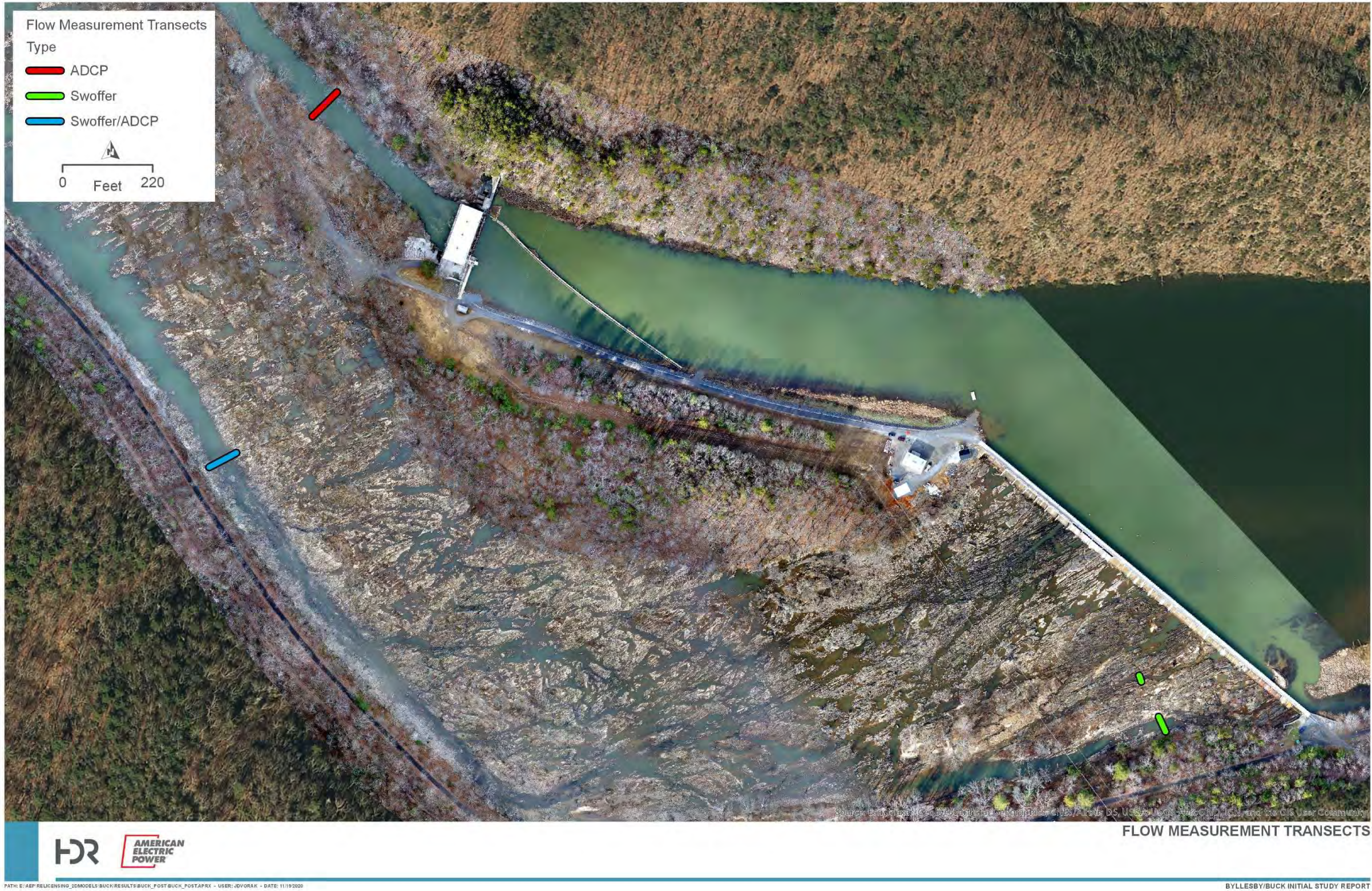
Figure 2-2. Flow Measurement Transects
