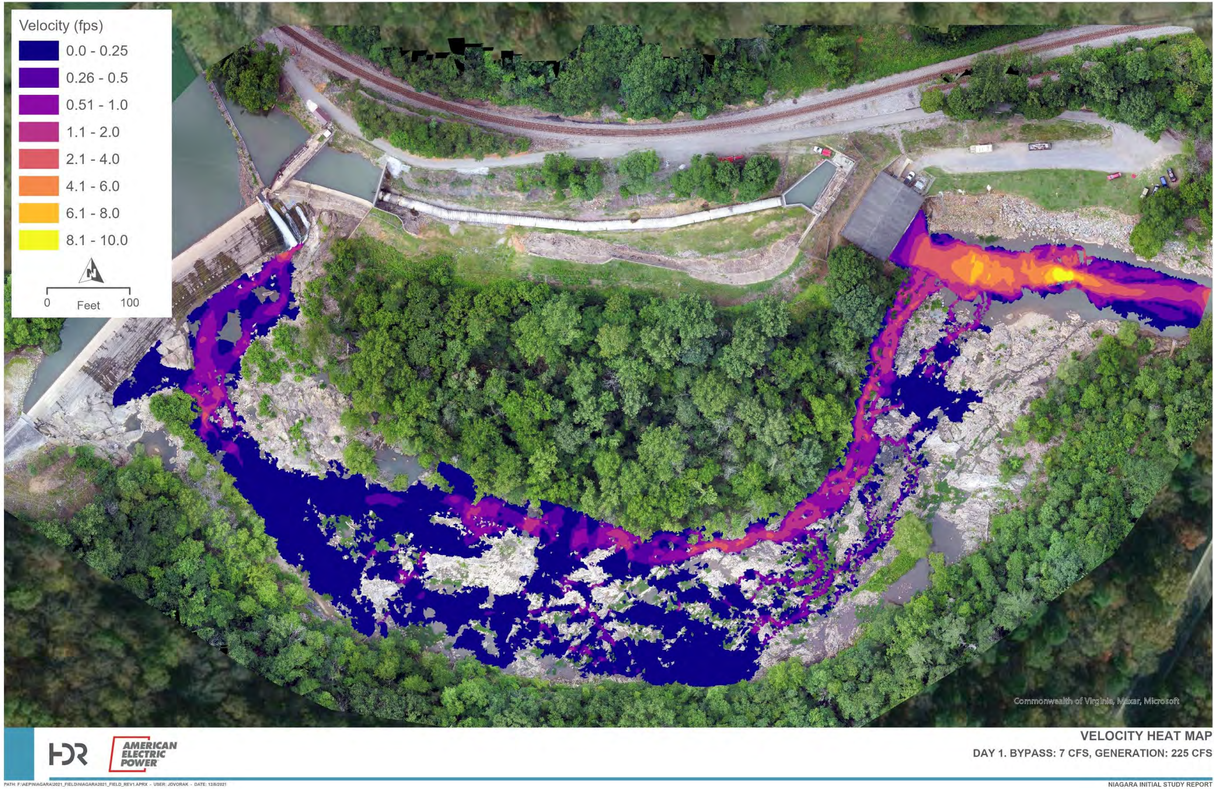
Figure 4-9. Velocity Heat Map – Minimum Flow
