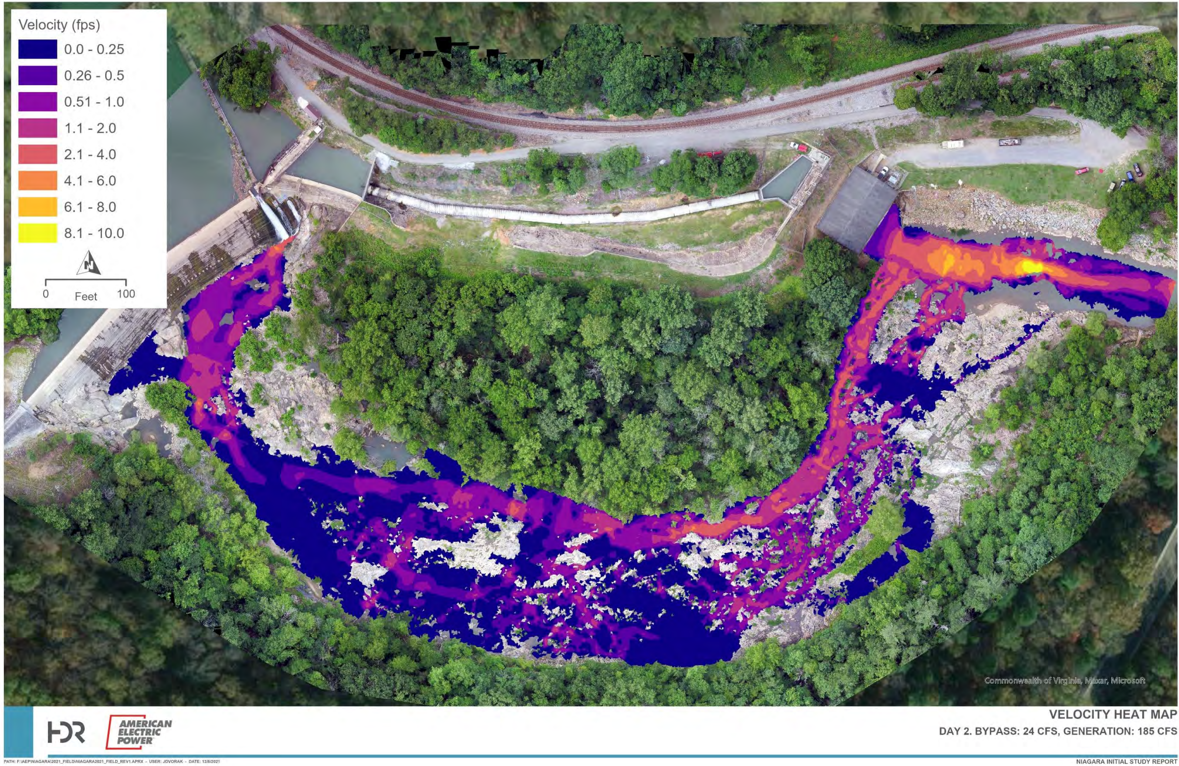
Figure 4-10. Velocity Heat Map – Low Flow
