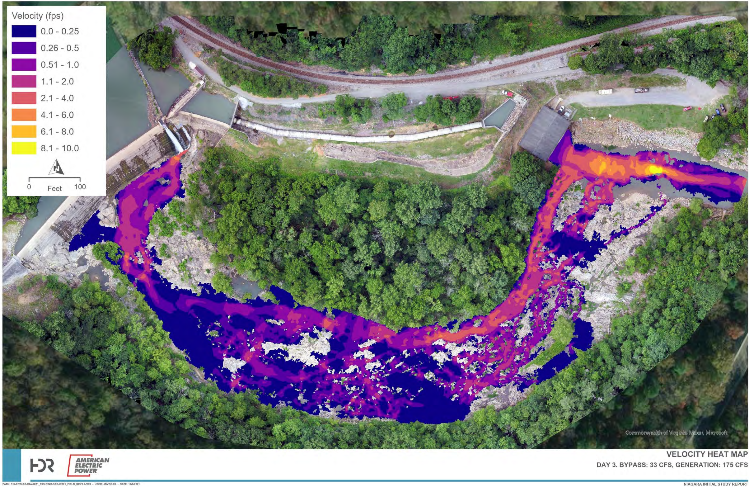
Figure 4-11. Velocity Heat Map – Middle Flow
