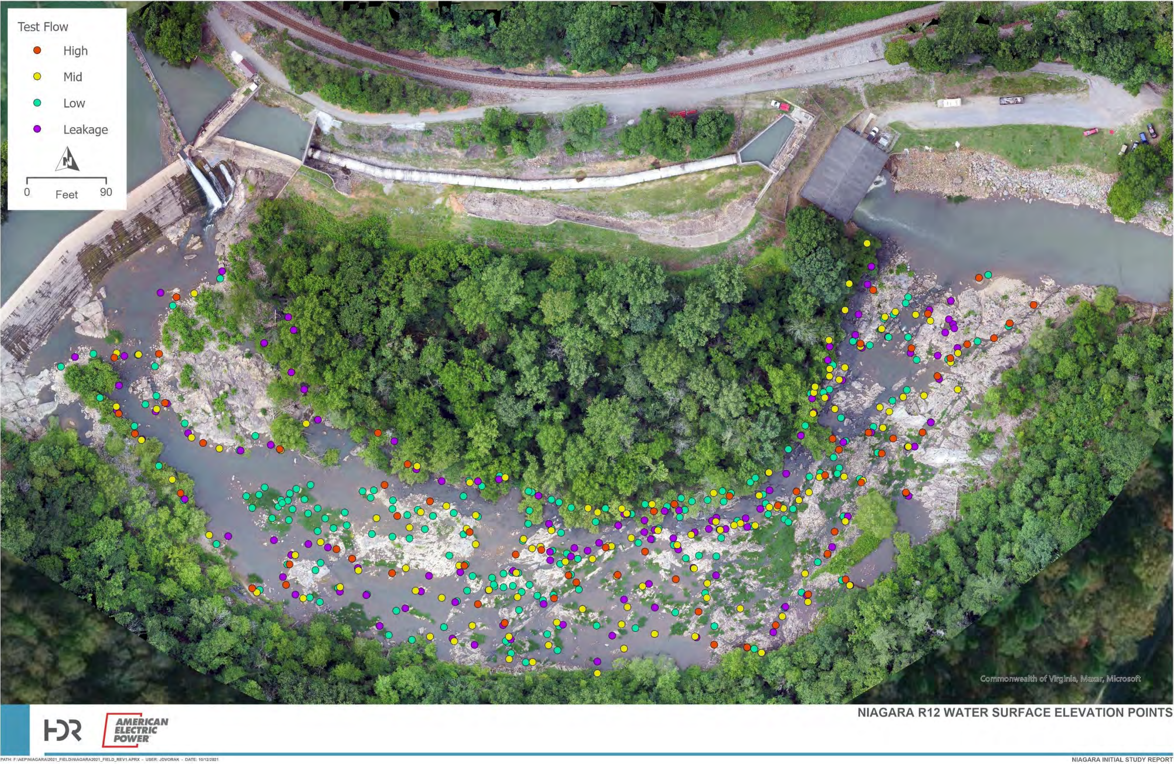
Figure 2-2. R12 GPS Water Surface Elevation Point
