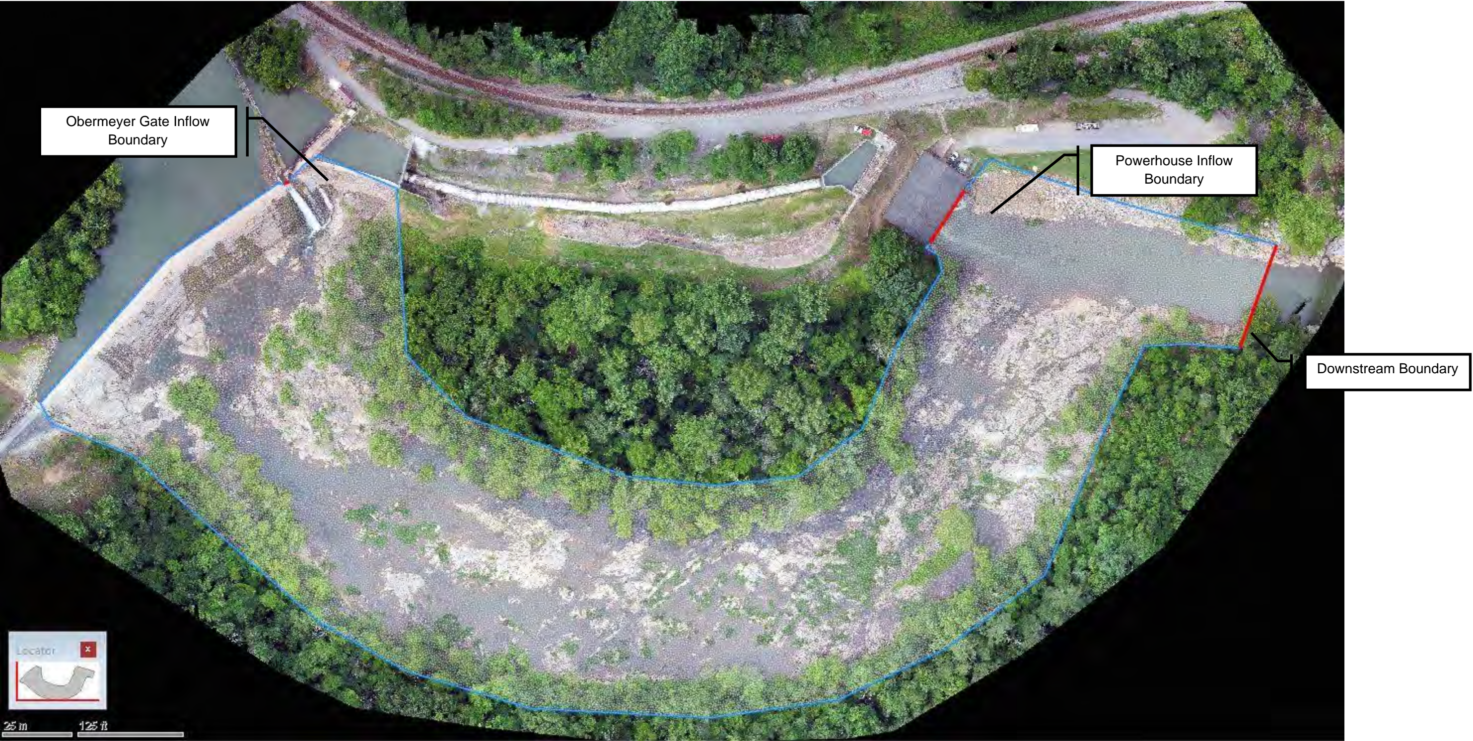
Figure 3-2. Extent of 2-D Zone and ICM Mesh (North is to the Top of the Figure)
