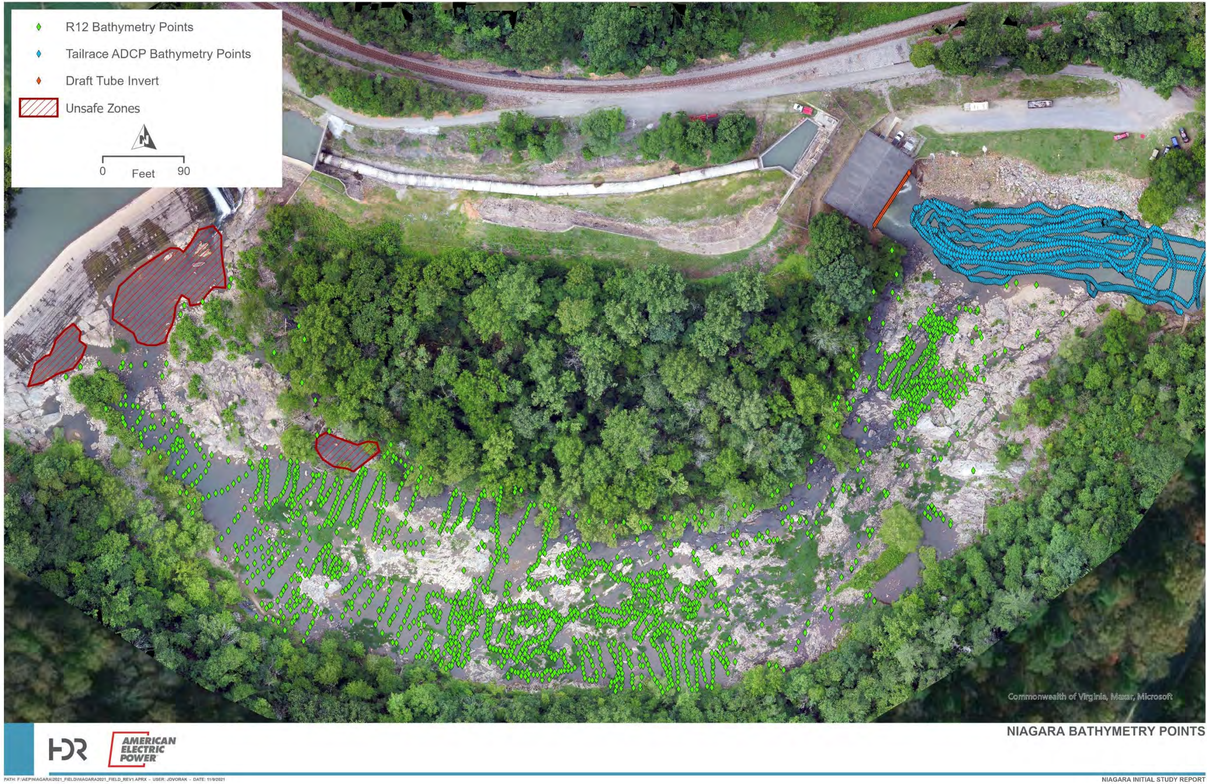
Figure 2-3. Collected Bathymetry Points
