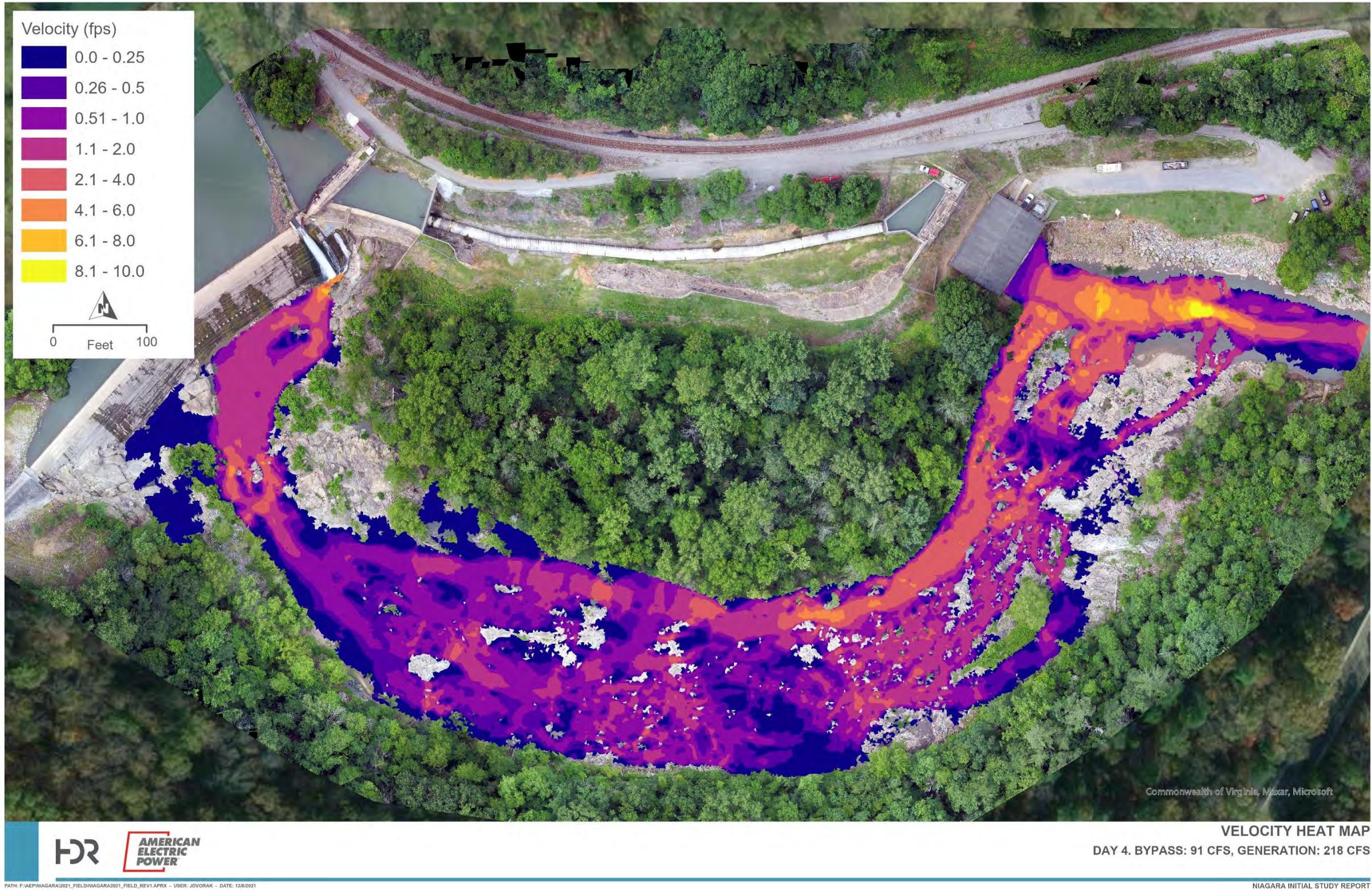
Figure 4-12. Velocity Heat Map – High Flow
