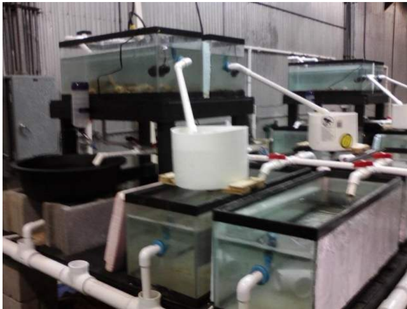
Photograph 1. Overall arrangement of the tank system used to hold adult darters and retain and rear their spawned larvae. The upper tanks held broodstock. The white buckets are the catch-buckets designed to passively capture larvae.
