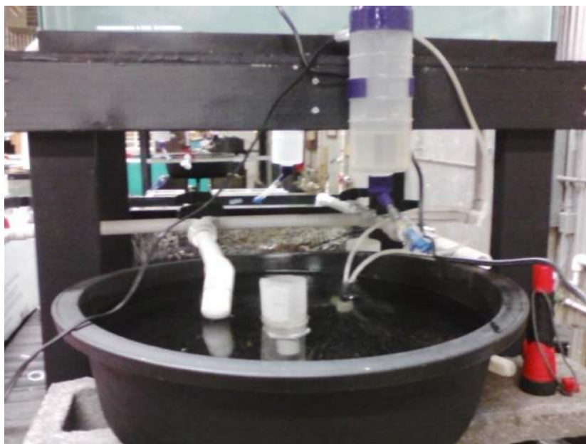
Photograph 2. Pelagic dish for rearing larvae. The sieve in the middle prevents larvae from flowing out. The bottle (upper right) is a drip-feeder that delivers food.
