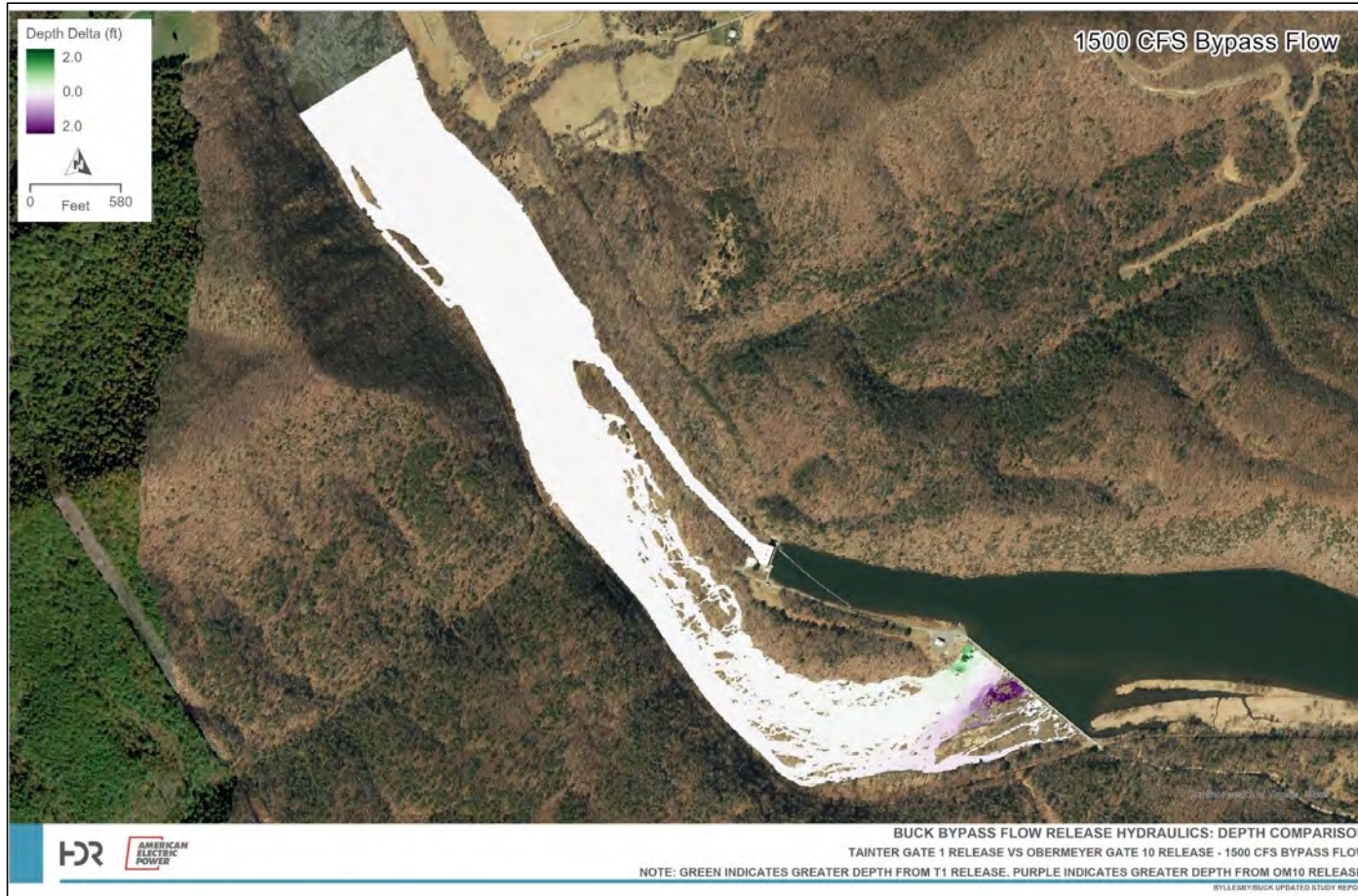
Figure E.9-8 Buck Bypass Reach Flow Release Hydraulics – Depth Comparison
