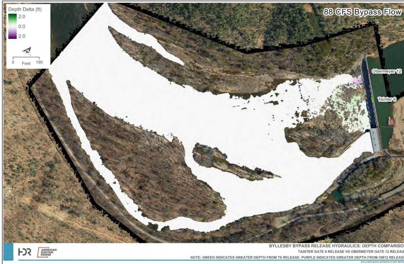
Figure E.9-4 Byllesby Bypass Reach Release Hydraulics – Depth Comparison
